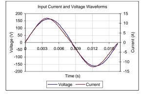
Input AC Current Waveform (ITHD = 5.52%, 50% Load)
