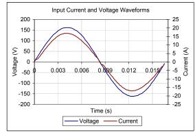
Input AC Current Waveform (ITHD = 3.99%, 50% Load)
