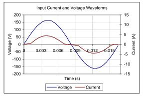
Input AC Current Waveform (ITHD = 25.48%, 50% Load)
