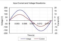
Input AC Current Waveform (ITHD = 7.67%, 50% Load)
