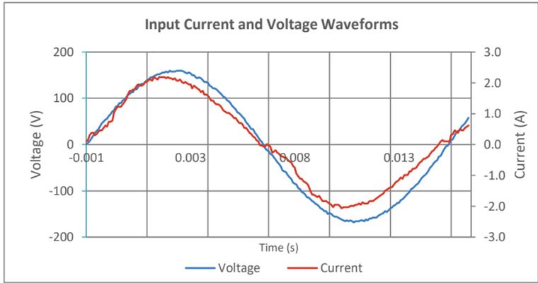
Input AC Current Waveform (ITHD = 9.76%, 50% Load)
