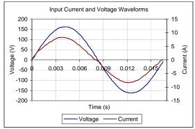
Input AC Current Waveform (ITHD = 6.95%, 50% Load)
