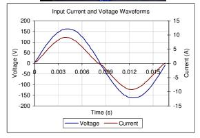
Input AC Current Waveform (ITHD = 13.7%, 50% Load)
