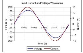
Input AC Current Waveform (ITHD = 5.38%, 50% Load)
