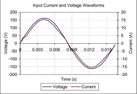
Input AC Current Waveform (ITHD = 5.33%, 50% Load)
