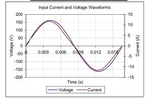
Input AC Current Waveform (ITHD = 6.04%, 50% Load)
