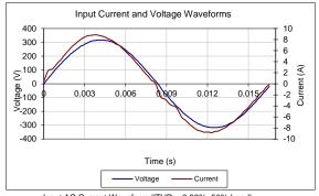
Input AC Current Waveform (ITHD = 3.89%, 50% Load)
